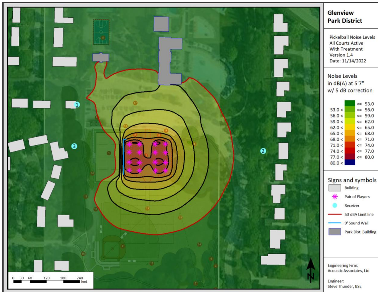
Figure 4 – Sound level contours around the proposed pickleball courts with mitigation
